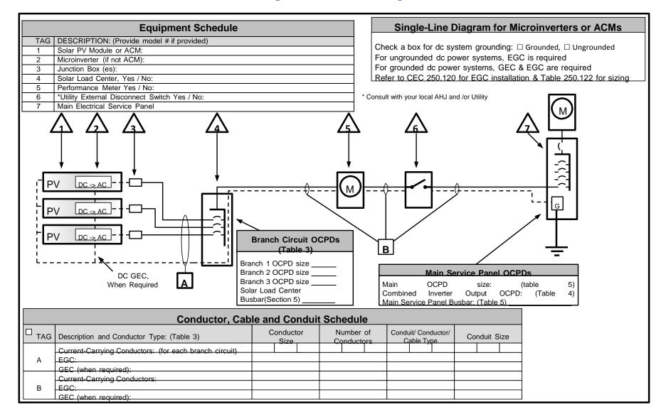
Equipment Grounding Conductor smaller than #6 gauge shall be protected a raceway or cable armor unless installed within hollow spaces of Framing members of buildings per CEC 250.120(C), 250.134 (B) exception #2 and 690.46.
