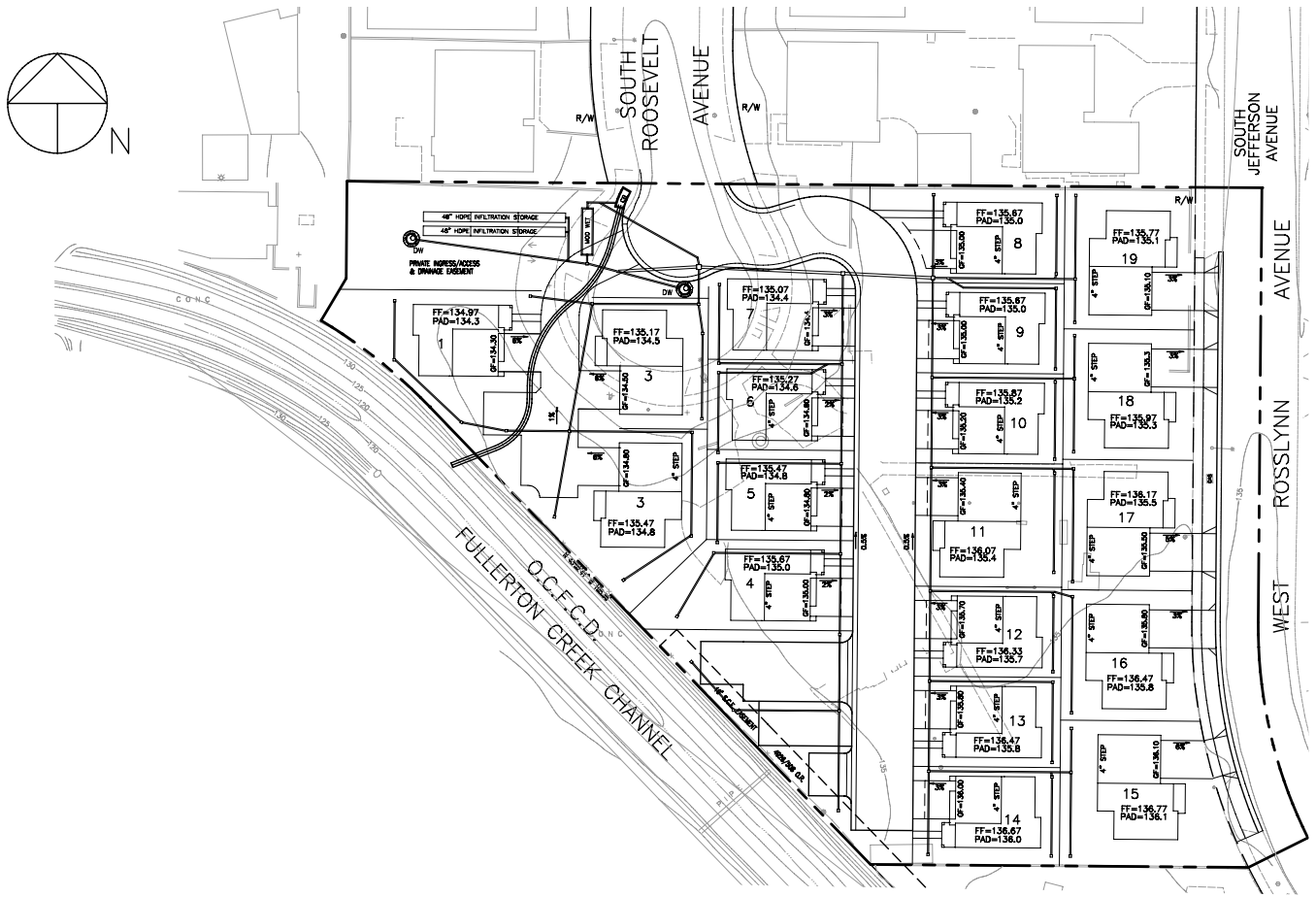
Figure 3.2 Preliminary Grading and Storm Drainage Plan
