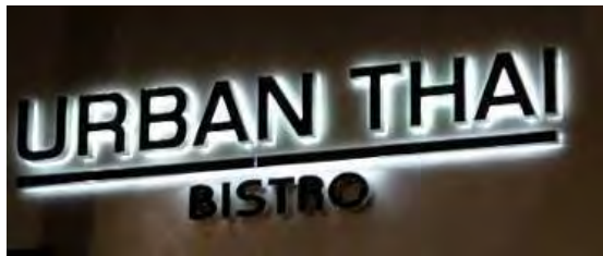
Back-lighting of cut-out letters and symbols that are mounted to the wall (allowed)
