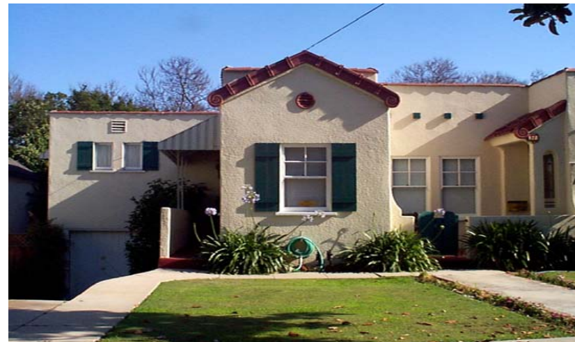
A residence on the 500 block of West Malvern Avenue: the shutters have the proper size and design for the windows of a Spanish Colonial Revival house.
